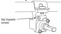
Turn the bypass screw on each control clockwise to the stop.
